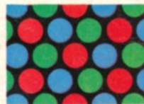
Magnified drawing of new Zenith Chromacolor picture screen
